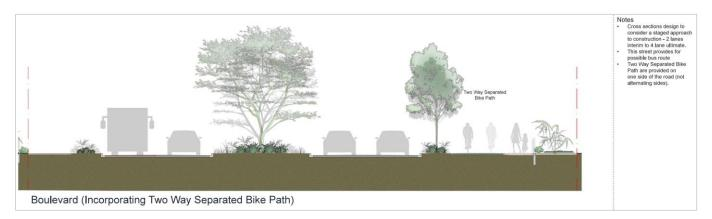
Figure 2: Cross sections for two way separated bike path<sup>7</sup>
