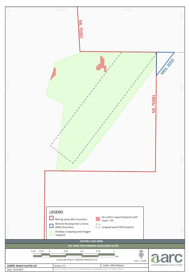
Figure 8: Inferred slopes >3% post-mining (MSEC [2022] predicted subsidence DEM)
