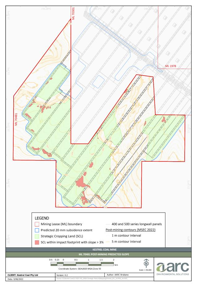
Figure 6: Inferred slopes >3% post-mining (MSEC [2022] predicted subsidence DEM)
