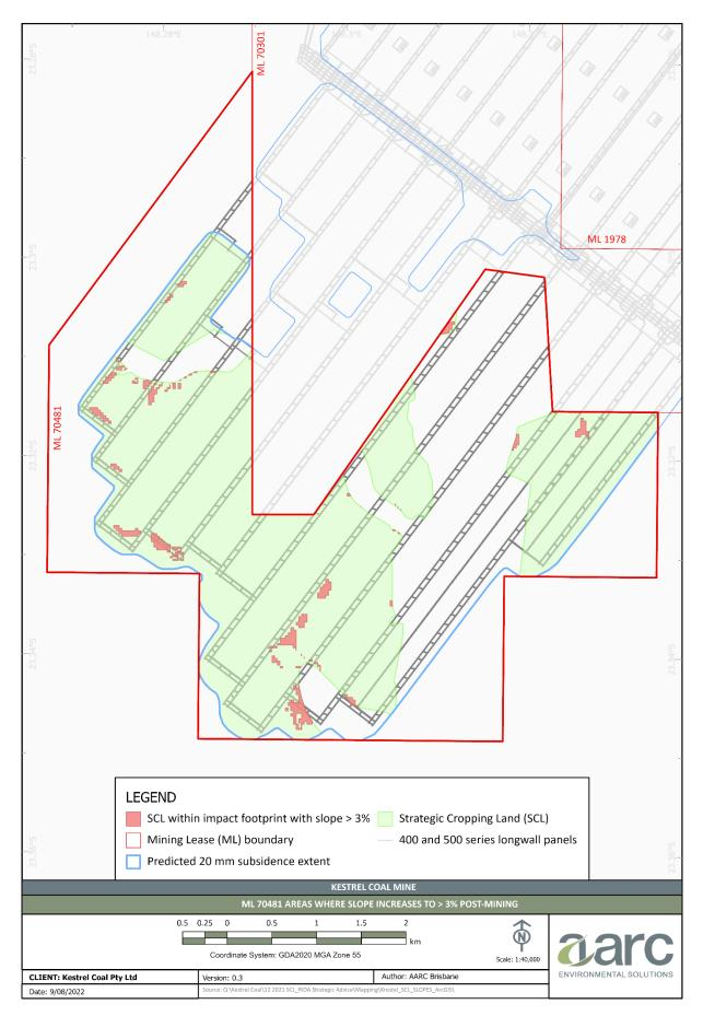
Figure 7: Inferred subsidence-induced slope changes to greater than 3%
