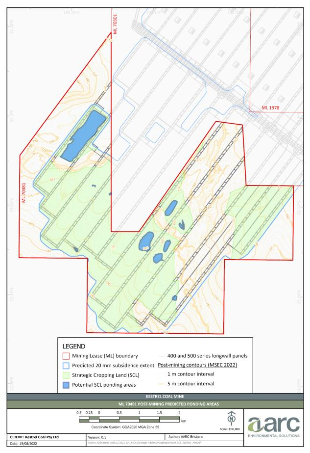
*Figure 8: Inferred ponding subsequent to subsidence*
