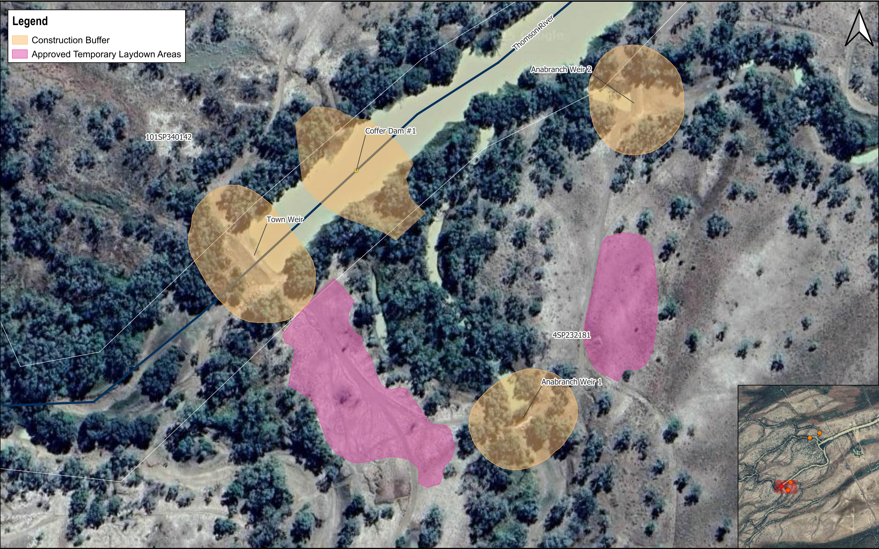
GLC00322_0007 Thomson River Weir RIDA Amendment Figure 2.2 Proposed Cofferd Dam #1 and Additional Town Weir Disturbance
