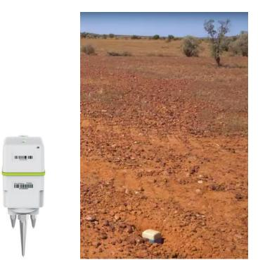
Plate 3.1 Example of a Passive Seismic Receiver Node and In-ground Placement
