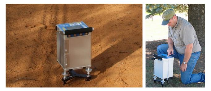
Plate 3.2 Example of a Ground Gravity Meter
